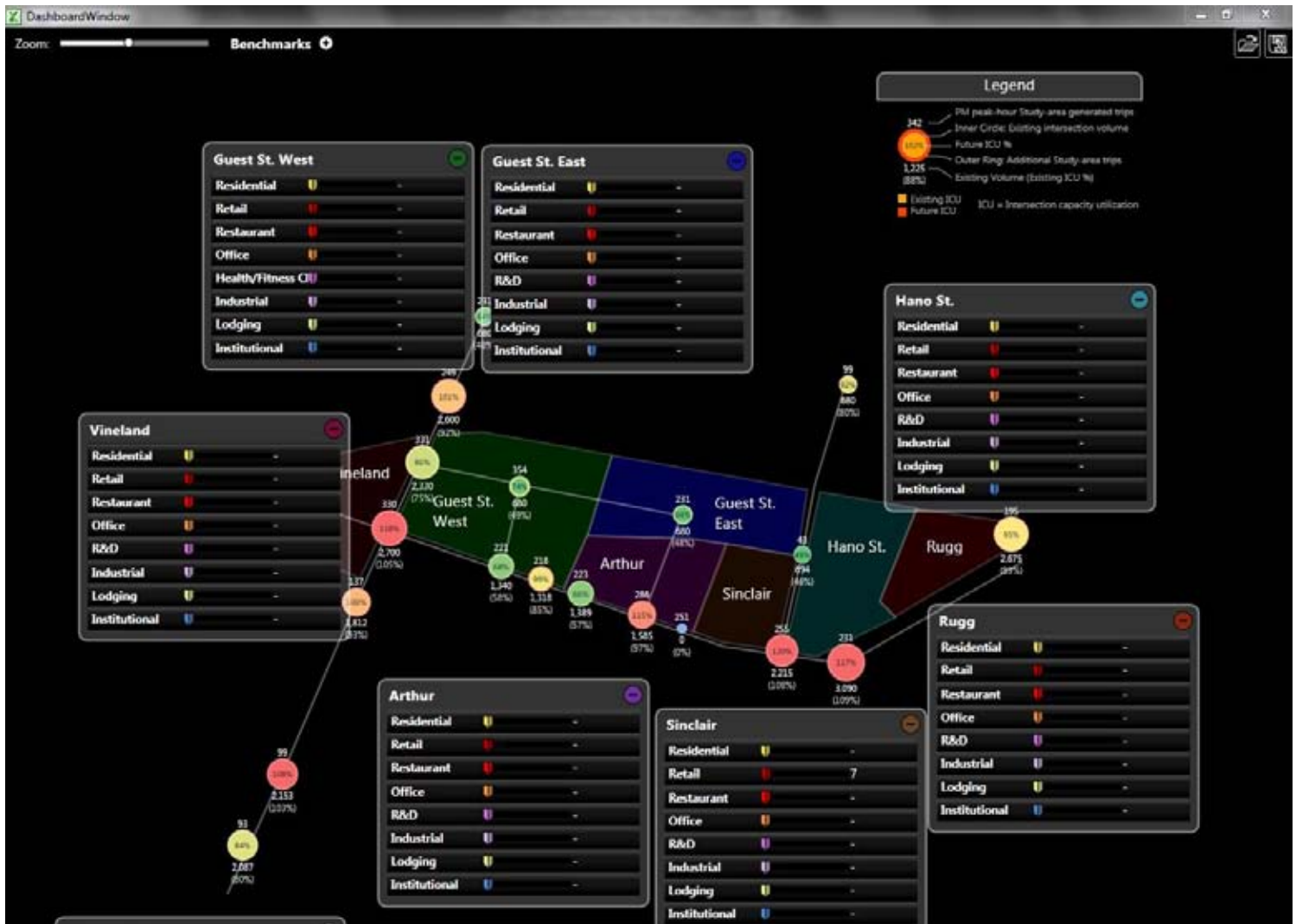
ILLUSTRATION OF TRANSPORTATION SOFTWARE USER INTERFACE THAT MODELS CONTEXT AREA TRAFFIC IMPACTS.
