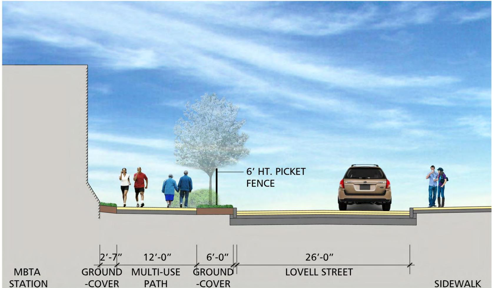
MULTI-USE PATH IN FRONT OF MBTA STATION CROSS SECTION
