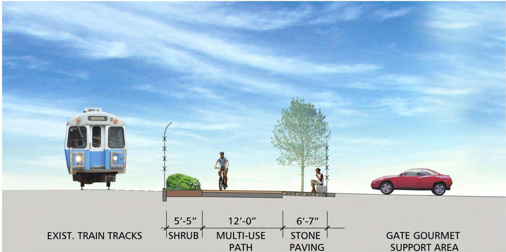
MULTI-USE PATH AT THE BACK OF GATE GOURMET SUPPORT AREA CROSS SECTION
