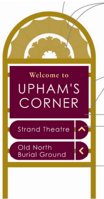
Four free standing light weight steel frame signs, surface mounted on existing concrete medians sidewalks
