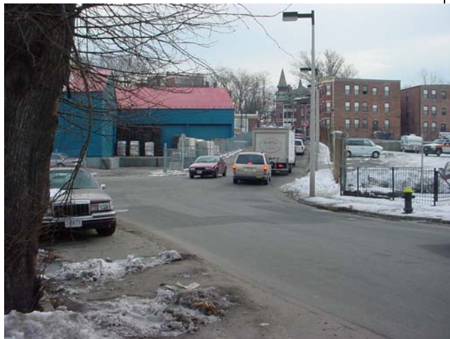
The Amory Street and Dimock Street Intersection. The red car facing the camera has a stop sign. There are no visible pavement markings. The intersection is difficult for pedestrians to cross safely.
