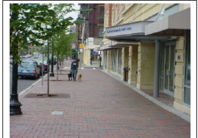
Street trees create a buffer between the walking zone and the roadway.
