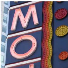
Channel Neon Tube Light is emitted by neon tubes mounted inside channels, creating a glow effect.
