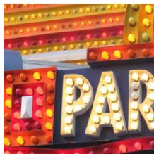
Exposed Incandescent Exposed bulbs mounted to the face of a sign create the illumination.
