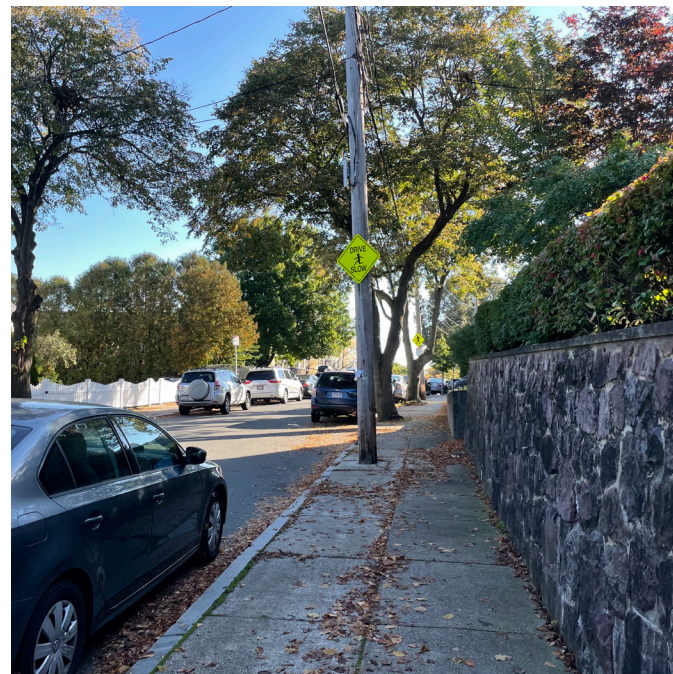
Many sidewalks in East Boston are narrow, and do not provide enough width for the Pedestrian Zone. New construction fronted by an inadequate sidewalk may be asked to set the building back to allow for the expansion of the sidewalk.
