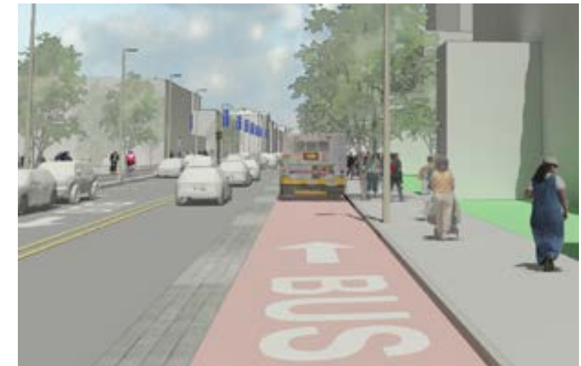
Figure 41. Conceptual drawing of potential "Complete Streets" improvements for Columbus Avenue, including bus rapid transit (BRT) elements, protected bicycle accommodations, improved sidewalks, and landscaping
