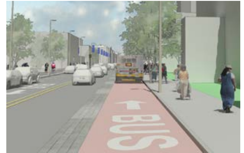
Figure 59. Conceptual drawing of potential "Complete Streets" improvements for Columbus Avenue, including landscaping, bus rapid transit (BRT) elements, protected bicycle accommodations, and improved sidewalks
