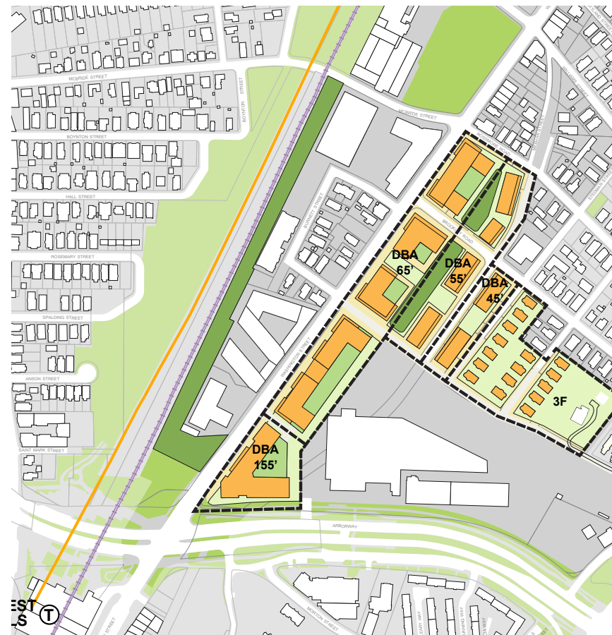
Figure 91. Conceptual plan drawing to provide details of the development scenarios in the Forest Hills focus area, with height zones
