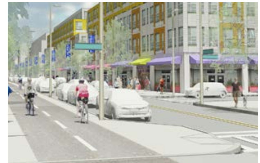
Figure 63. Conceptual drawing of potential "Complete Streets" improvements for Washington Street, including landscaping, protected bicycle accommodations, and improved sidewalks
