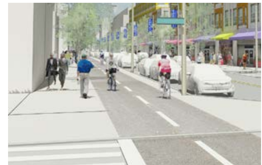
Figure 45. Conceptual drawing of potential "Complete Streets" improvements for Washington Street, including landscaping, protected bicycle accommodations, and improved sidewalks
