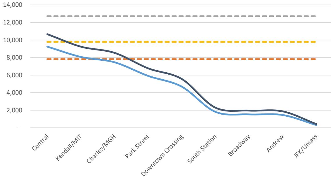
**Figure 5-13 Red Line PM Peak Hour Outbound Loads & Capacity**
