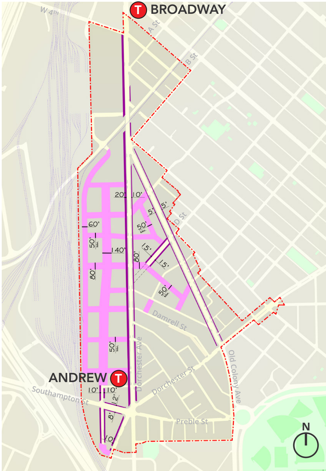
Figure 148. Conceptual diagram of property line setback requirements for creation of R.O.W.s. Exact location and widths of R.O.W.s to be determined by a future transportation study.
