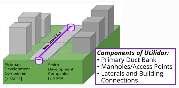
The BPDA presented a design scenario where two developers constructing along the same new street were recommended to build a Telecom Utilidor to meet the telecommunications needs for their future build-outs. The scenario challenged participants to identify ways to partner in the design, construction, payment, and operations of a shared asset that would benefit both them and their future tenants.
