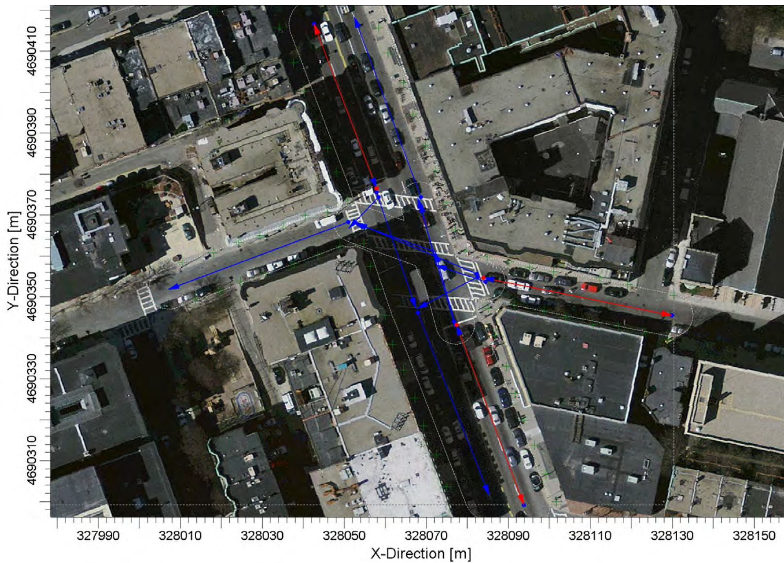
Figure 12.6-13 Link and Receptor Locations for CAL3QHC modeling of Intersection 2: the intersection of Massachusetts Avenue, Haviland Street, and Belvidere Street
