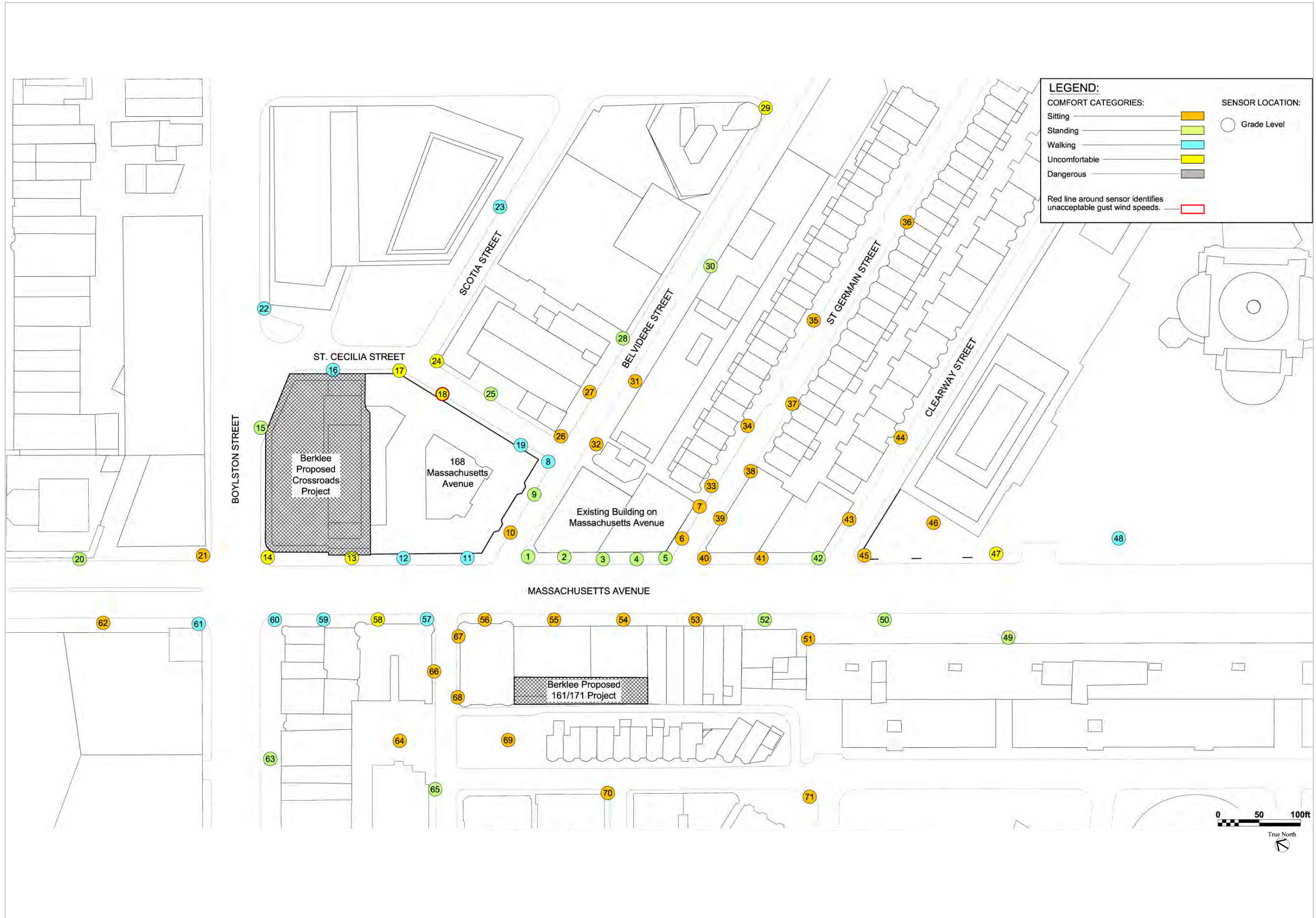
Figure 12.6-7 Pedestrian Wind Conditions - No Build
