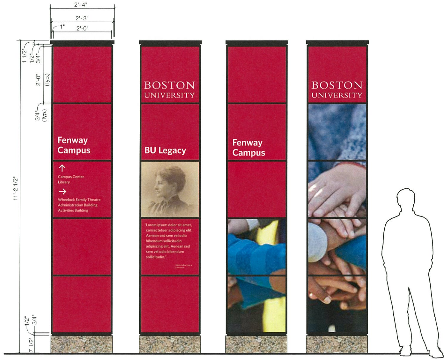
A: Directional Panel 1/2" = 1' - 0" B: Legacy Panel C: Image Panel D: Image Panel
