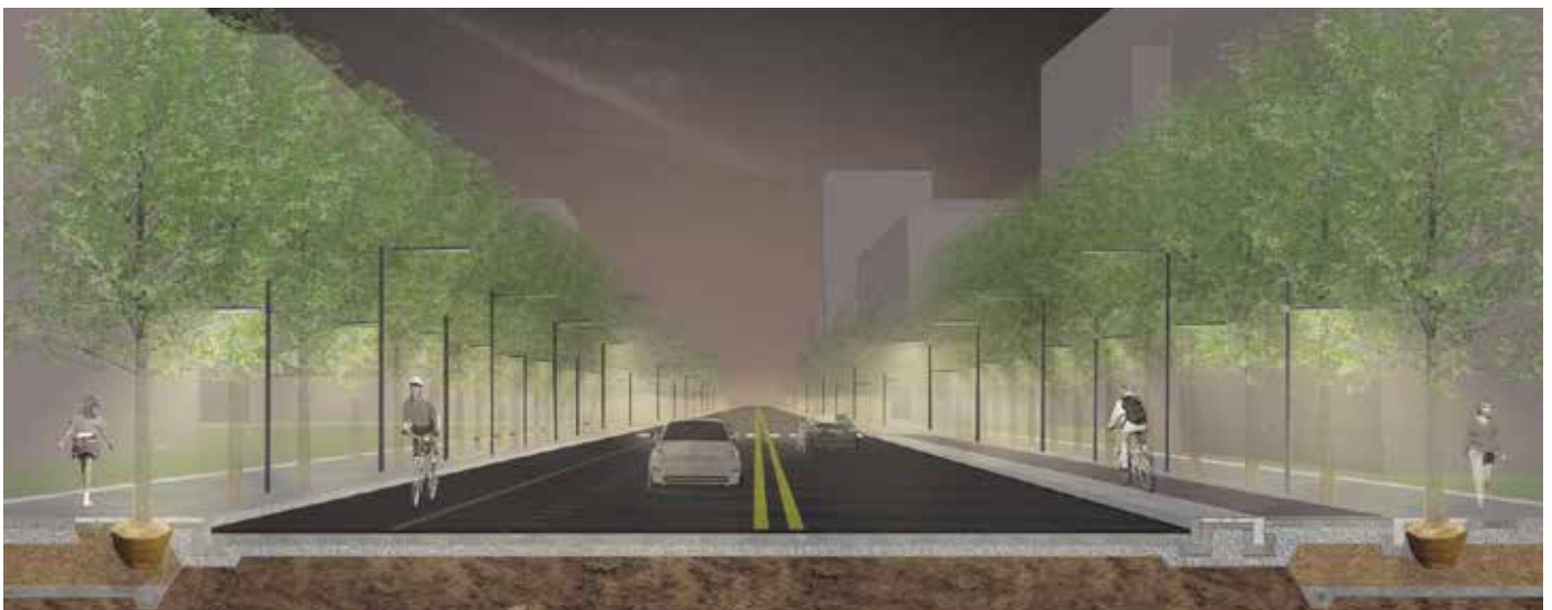
Dual-Height Lighting Along Western Avenue
