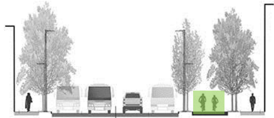
Stadium Rd – Curb Level Two-Way Path
