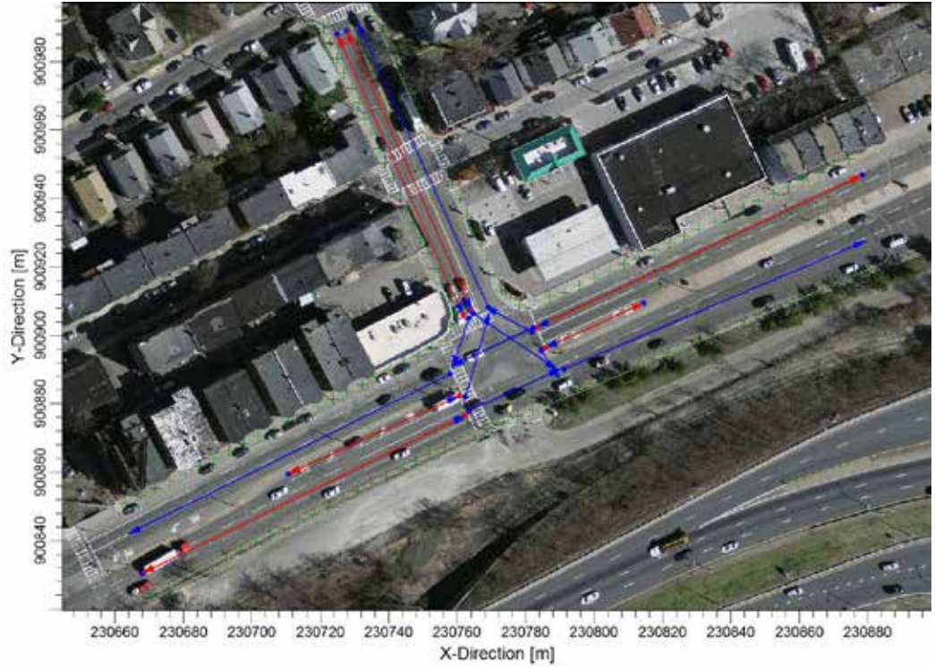
Figure 43: Link and Receptor Locations for CAL3QHC Modeling, Cambridge Street & North Harvard Street
