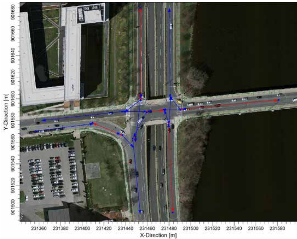
Figure 45: Link and Receptor Locations for CAL3QHC Modeling, Soldiers Field Road & Western Avenue
