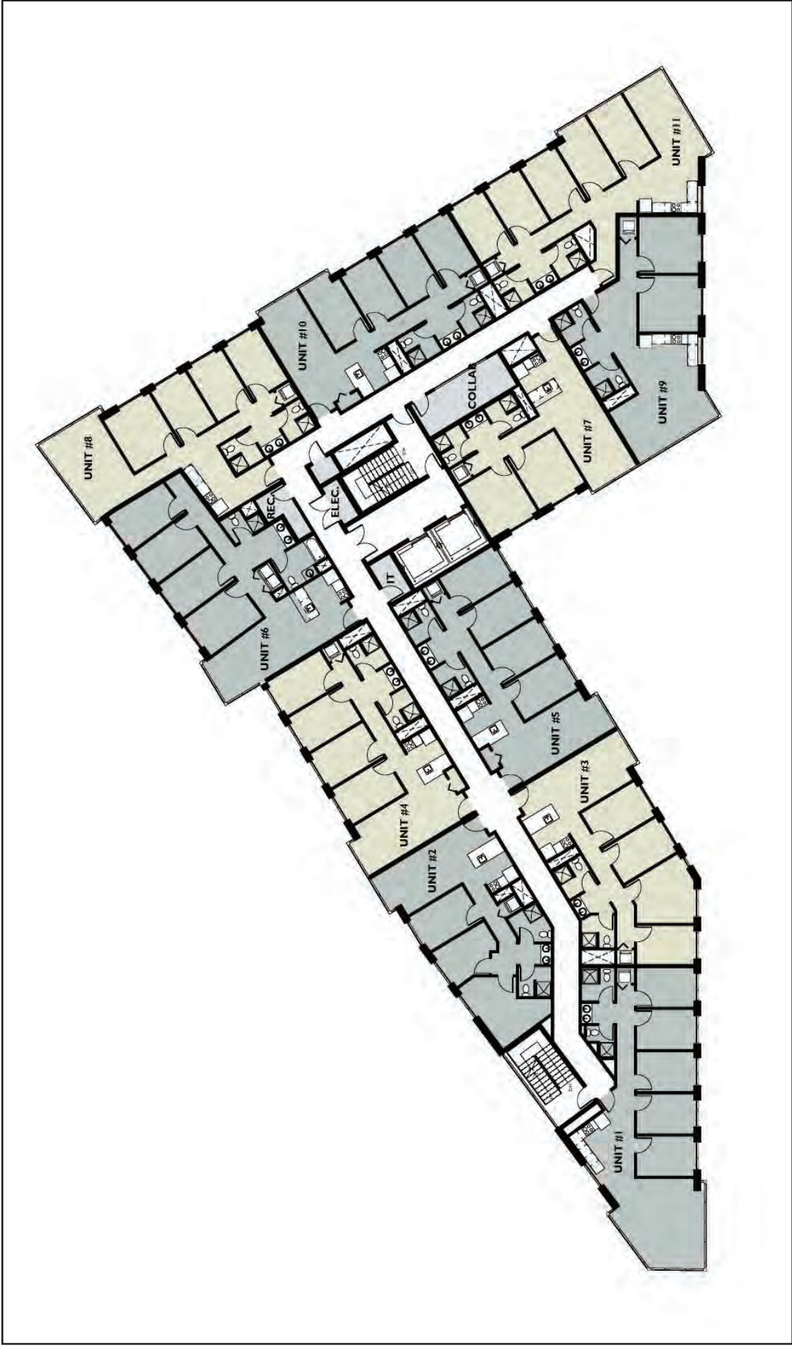
Figure 2-6 Typical Upper Level Floor Plan Source: Beacon Architectural Associates, 2012
