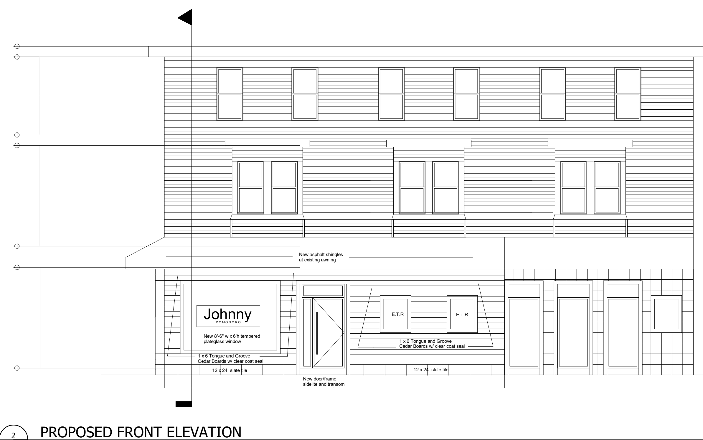
2 A8-2 PROPOSED FRONT ELEVATION 3/16" = 1'-0"
