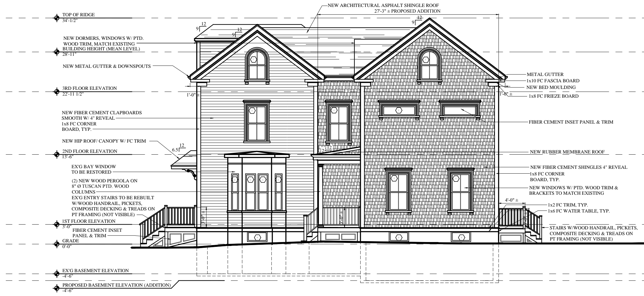
1 PROPOSED RIGHT ELEVATION 1/4" = 1'-0"
