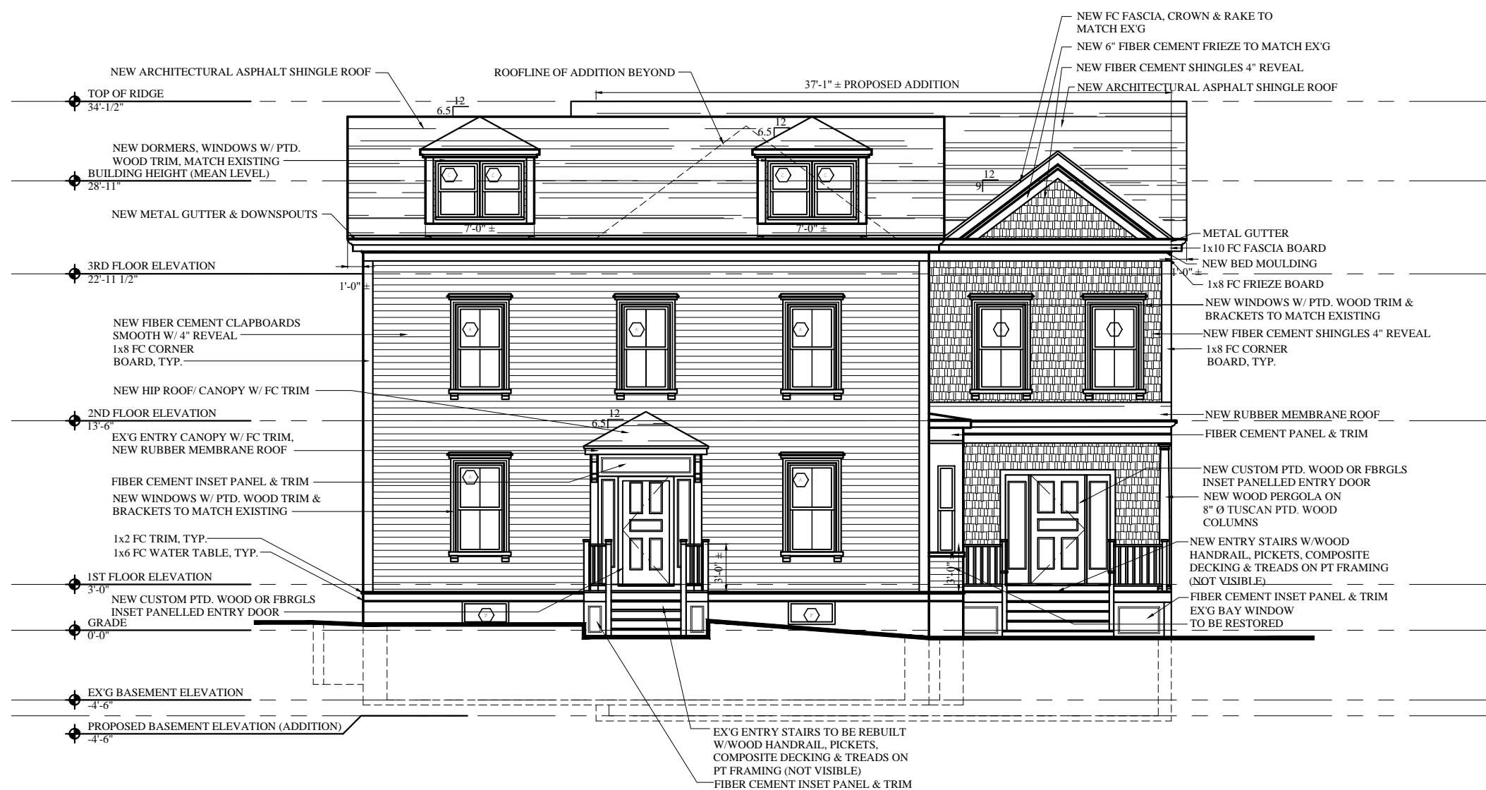
1 PROPOSED FRONT ELEVATION 1/4" = 1'-0"
