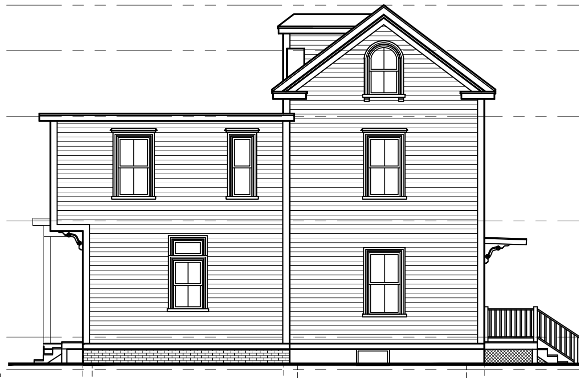
2 EXISTING LEFT ELEVATION 1/4" = 1'-0"
