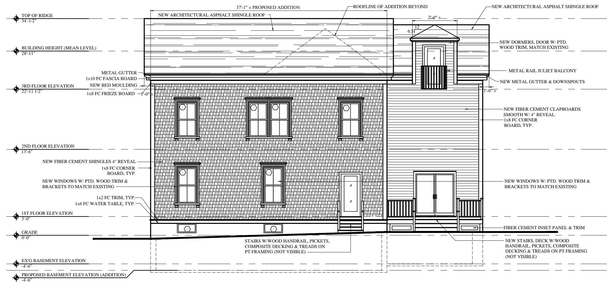
1 PROPOSED REAR ELEVATION 1/4" = 1'-0"
