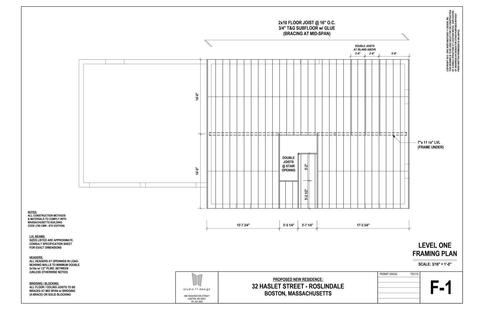
2x10 JOISTS @ 16" O.C. (BRACING AT MID-SPAN)
