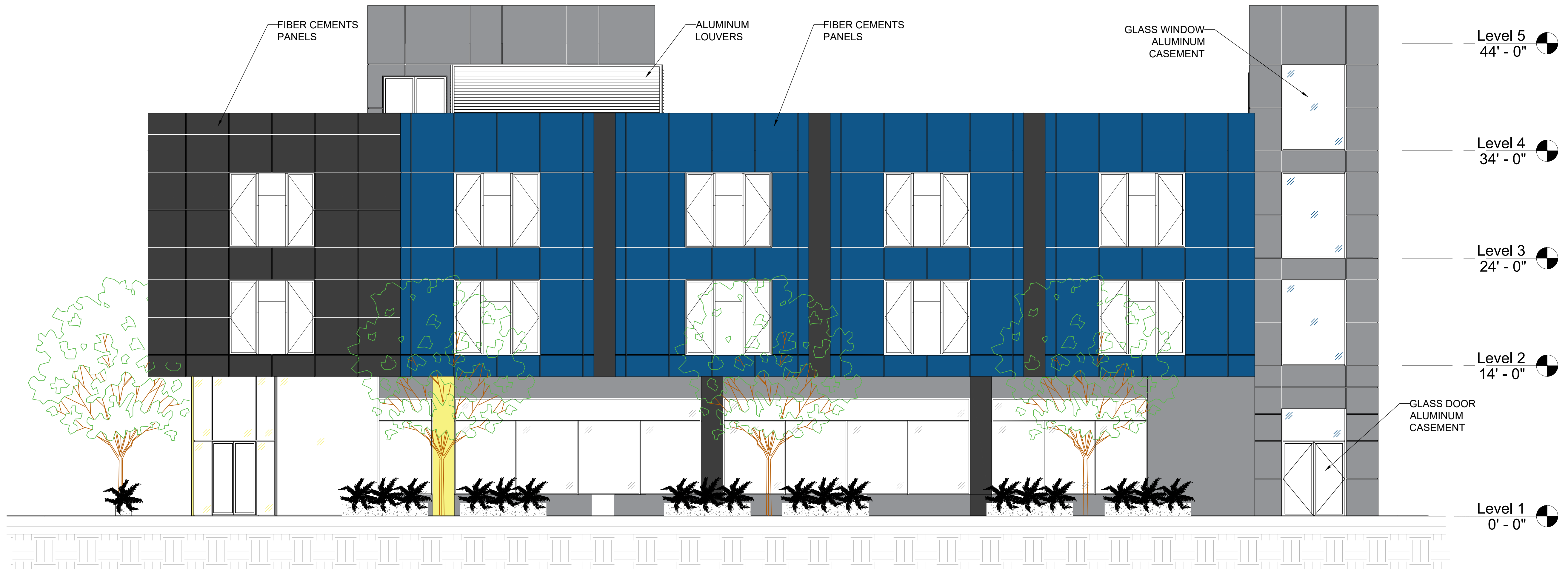
1 A-2.0 PROPOSED RIGHT ELEVATION SCALE: 3/16"=1'-0"
