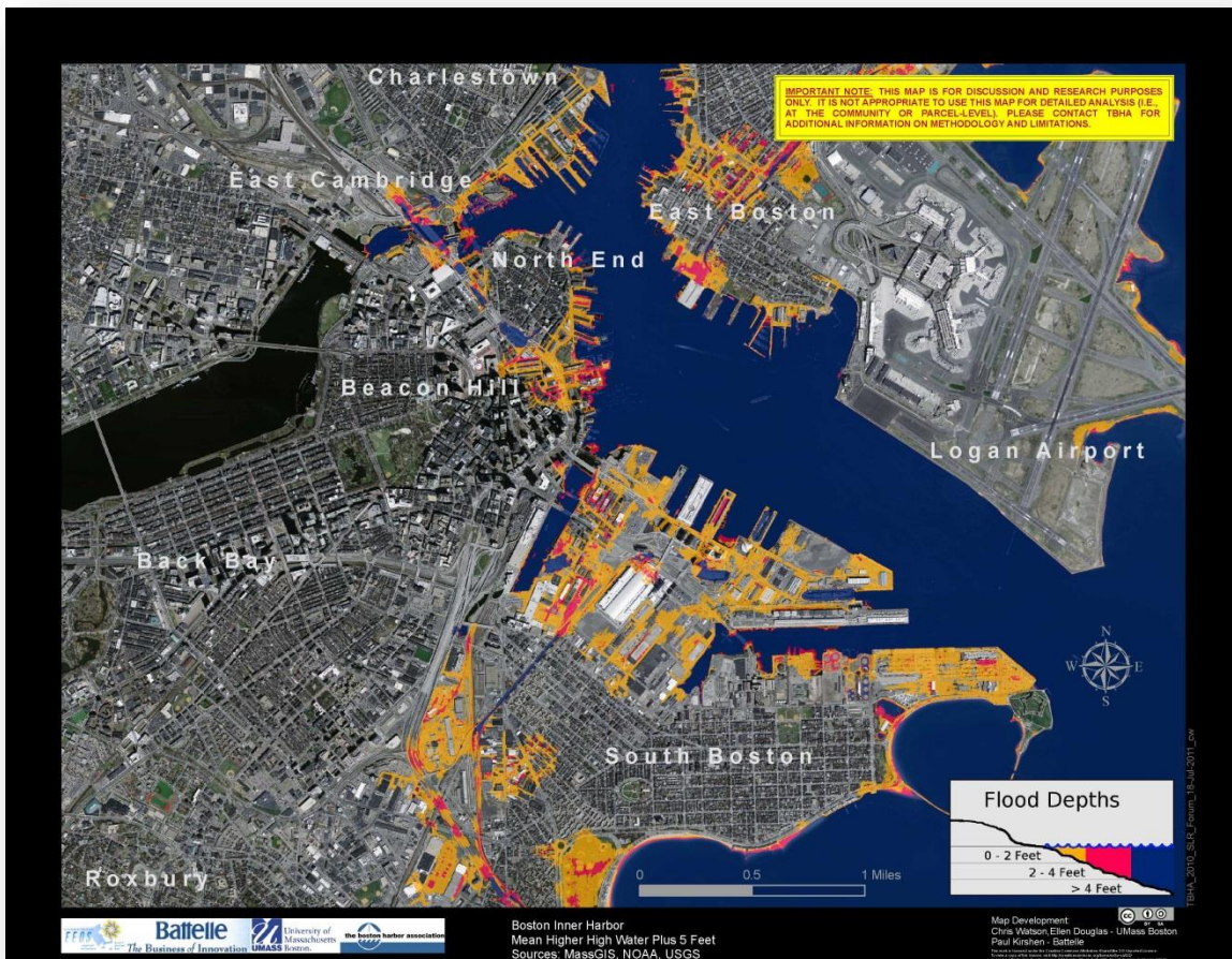
Figure 1-2. Potential flooding in Boston due to an extreme storm surge (5 ft) on top of spring tide. Source: www.tbha.org .
