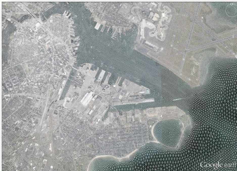
Figure 4-9. High resolution mesh grid in the vicinity of downtown Boston.
