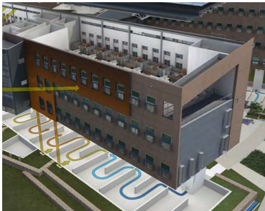
(top) Unstable soil conditions required the provision of a crawl space under the NREL Research Support Facility. The design team recognized this condition as an opportunity; the crawl space functions as part of the HVAC system, precooling and preheating air year round to reduce energy demand and therefore costs.
