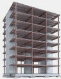
Concrete With Steel Frame
