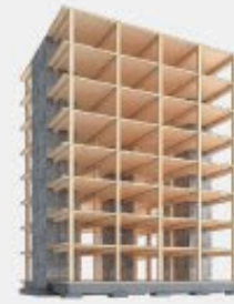
Timber 2 Post, Beam, & Plate
