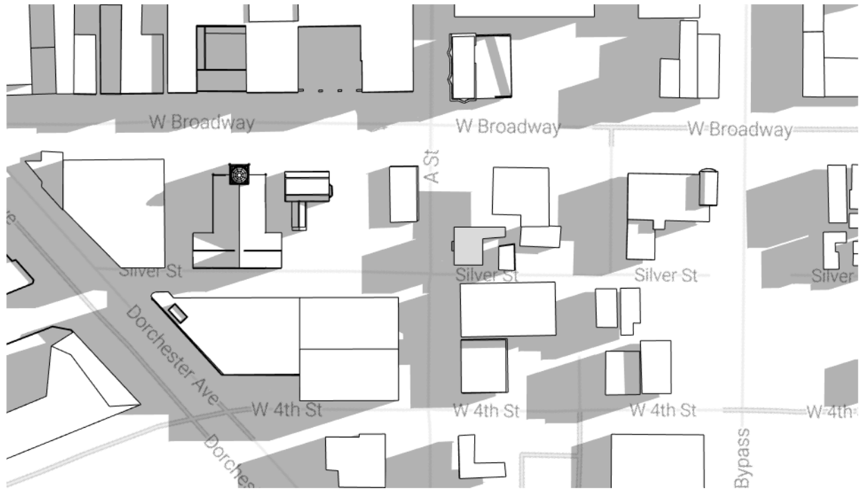
① Phase: Existing Sun Date: 3/21 Sun Time: 9AM Sun Altitude: 23° Sun Azimuth: 113°
