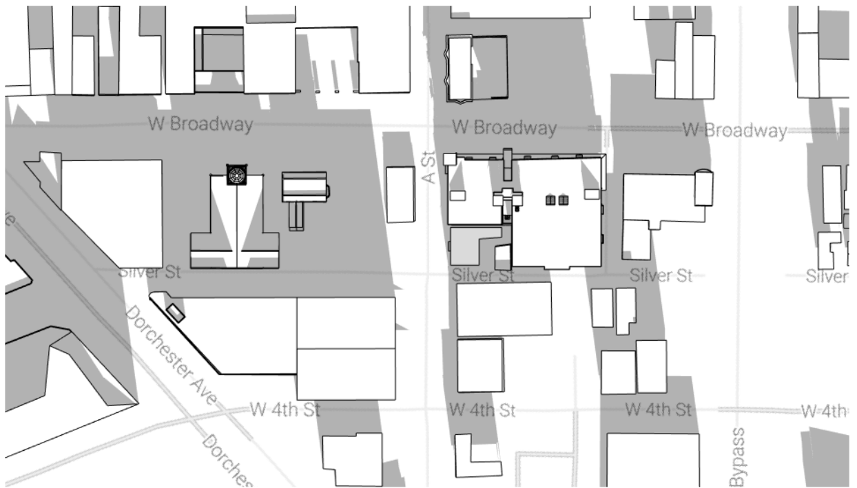
2 Phase: New Construction Sun Date: 12/21 Sun Time: 3PM Sun Altitude: 17° Sun Azimuth: -147°
