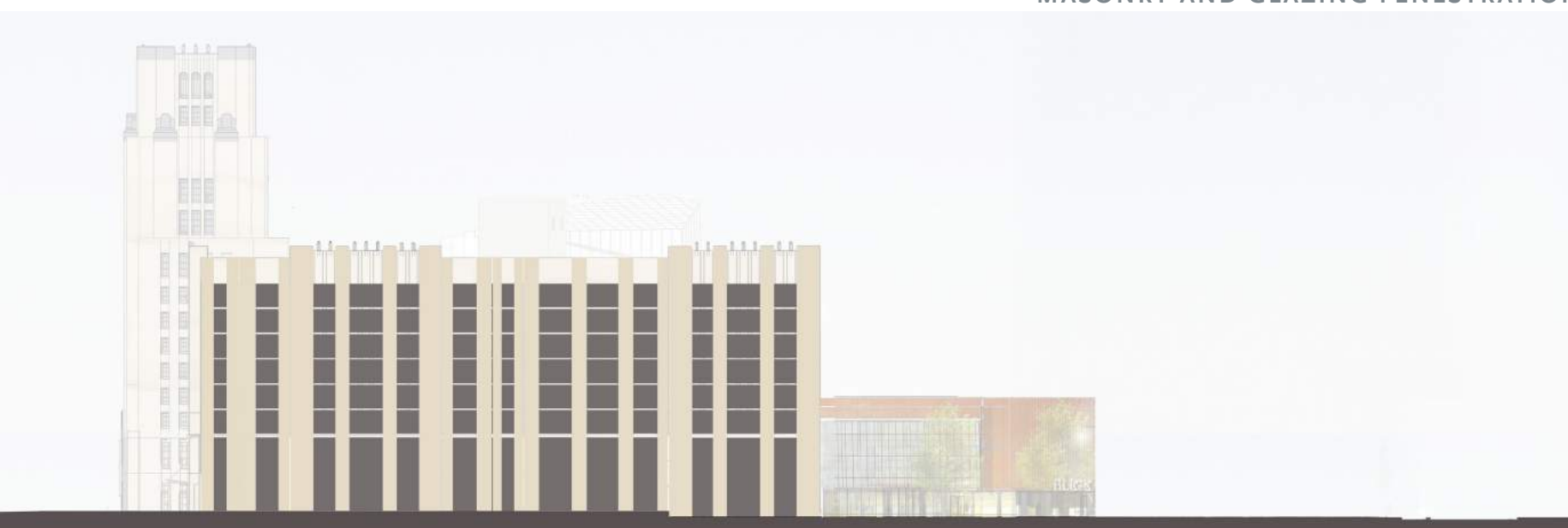
VERTICAL MASONRY AND GLAZING WITH SPANDRELS REMOVED
