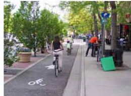
Planters, greenery, and special paving provide a visual as well as a physical buffer.
