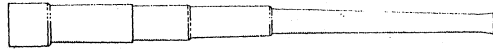
Period 3 (1900s-1920) - 6-inch quick-firing breech loader (Mark VII) firing a 100-pound exploding shell over a distance of 12,000 yards.
