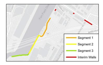
It also includes interim flood walls at the west end of Necco Court and beneath Summer Street at A Street and West Service Road. These would only be installed temporarily when major coastal flooding events are forecasted. The tops of these structures will be 1.5 feet higher than the FEMA 1% flood elevation. Interim flood walls will become redundant once flood control systems are constructed along other vulnerable segments of the South Boston waterfront over the next 10-20 years.
