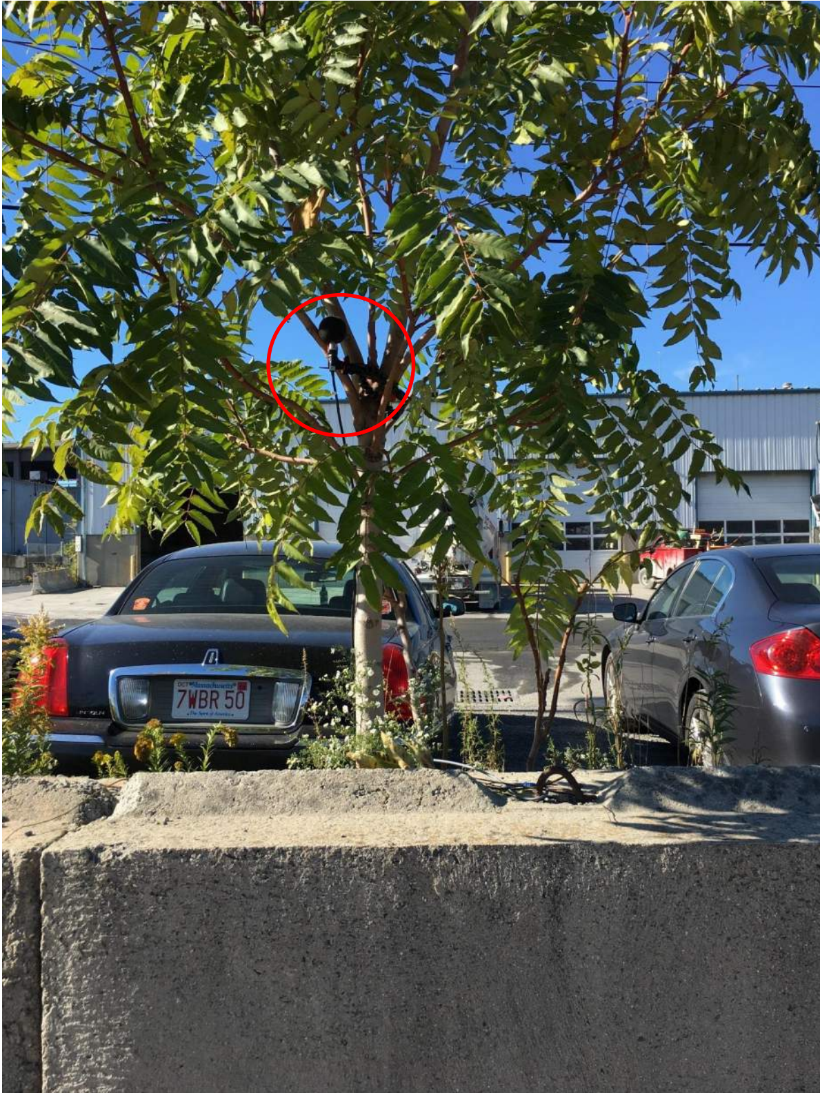
Photograph of Acentech logging Sound Level Meter as installed at Location #3. Microphone at red circle.
