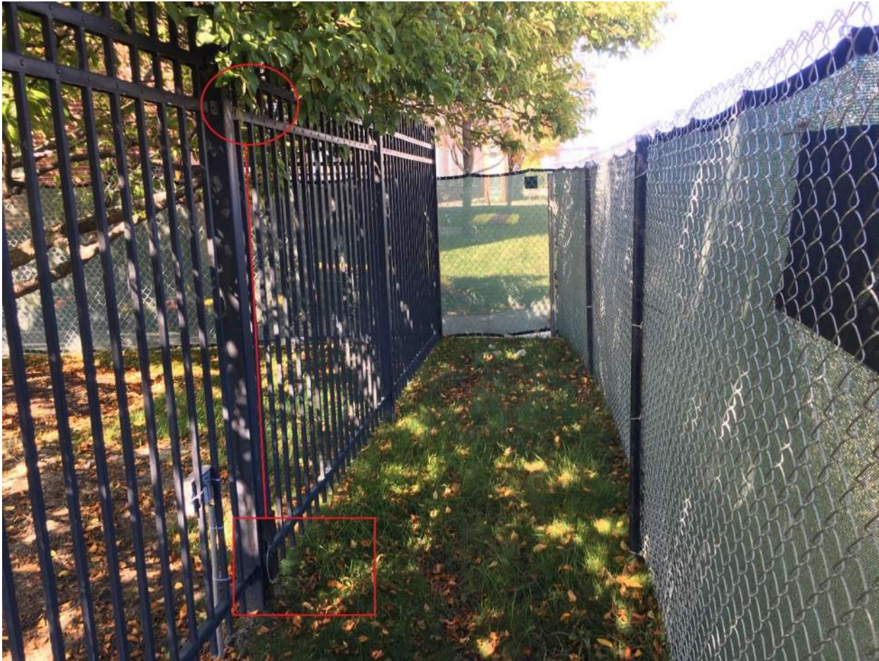
FIGURE 2: Location #1 between existing and construction fences. Red marks indicated the microphone (oval) and the instrumentation & battery pack (rectangle).
