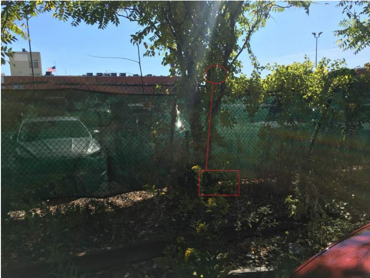
FIGURE 4: Location #2 with microphone (oval) located off tree branch. Leaves around microphone to be removed. Instrumentation to be located behind tree trunk and fence.
