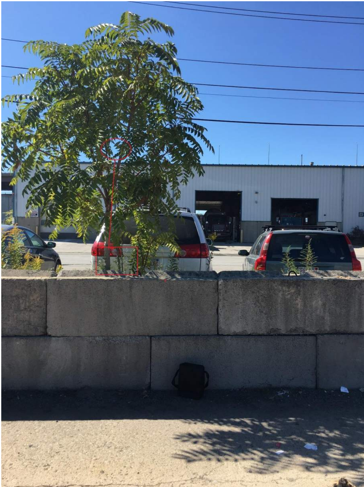
FIGURE 5: Location #3 microphone (oval) located off tree branch. Leaves around microphone to be removed. Instrumentation to be located on the opposite side of the concrete block on the ground.
