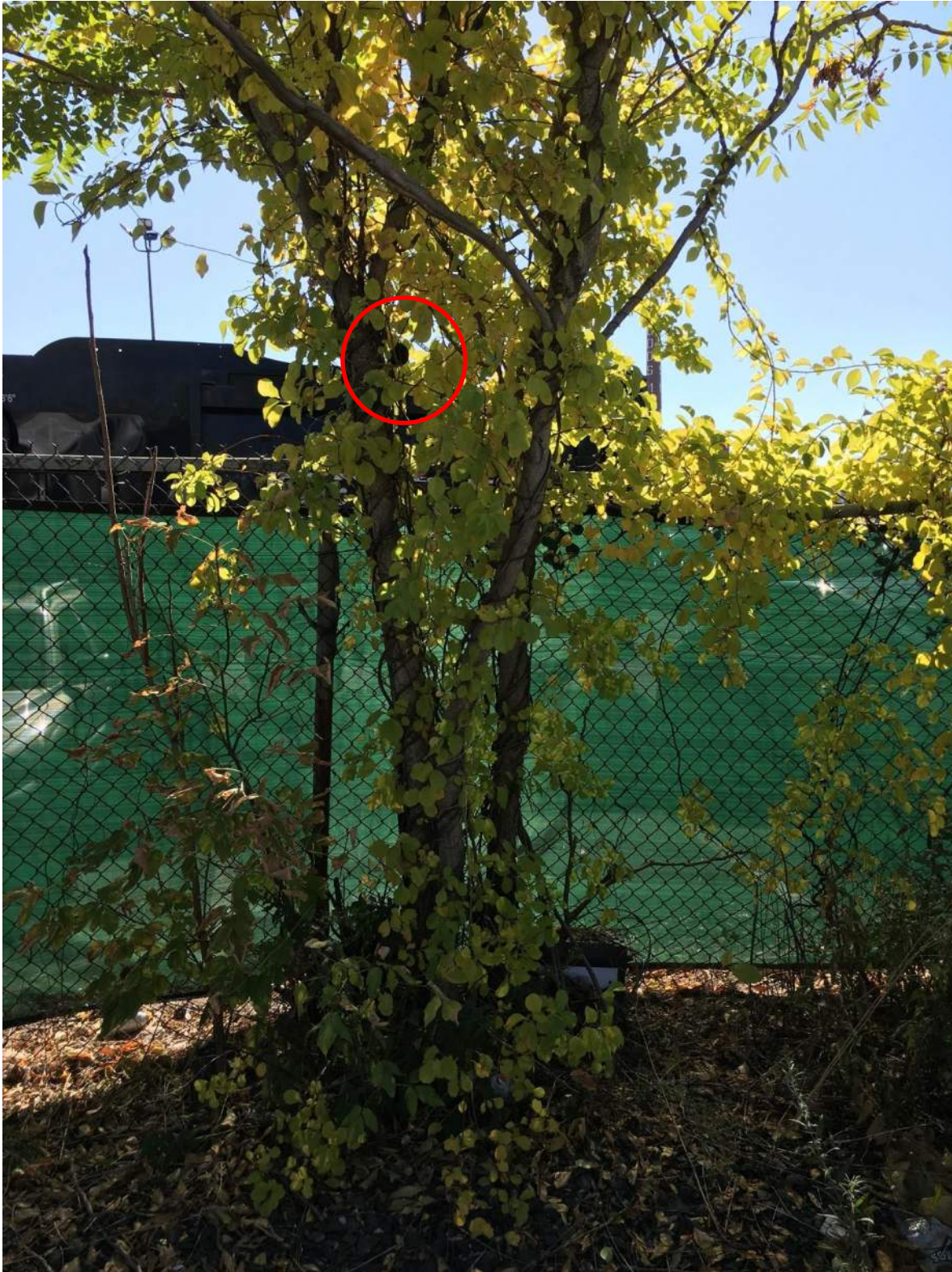
Photograph of Acentech logging Sound Level Meter as installed at Location #2. Microphone at red circle.
