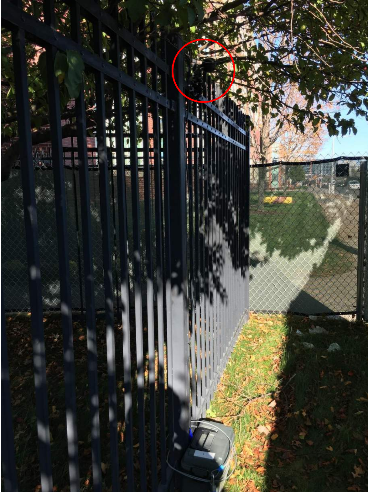
Photograph of Acentech logging Sound Level Meter as installed at Location #1. Microphone at red circle.
