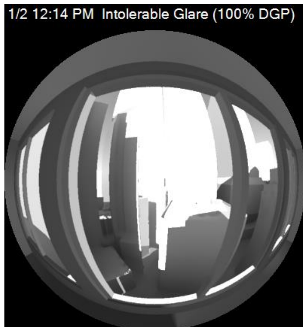
Figure 4 – DGP with new Winthrop Square Tower at model office location in Fig. 2.
