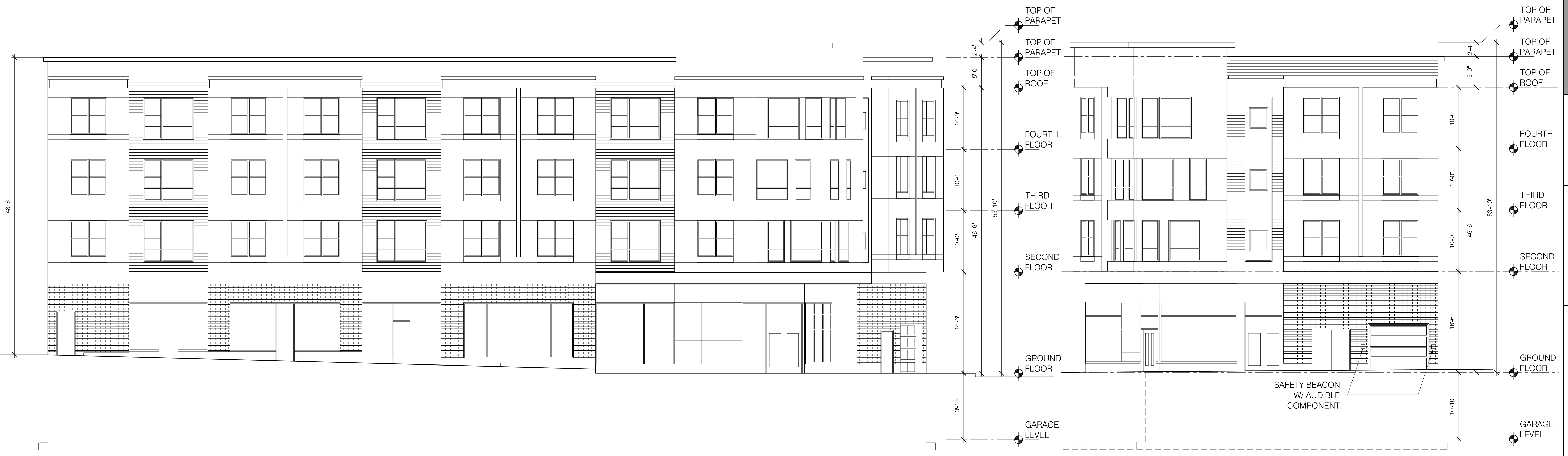
1 EXTERIOR ELEVATION - BLUE HILL AVENUE SCALE: 1/8" = 1'-0" 0' 4' 8' 16'
