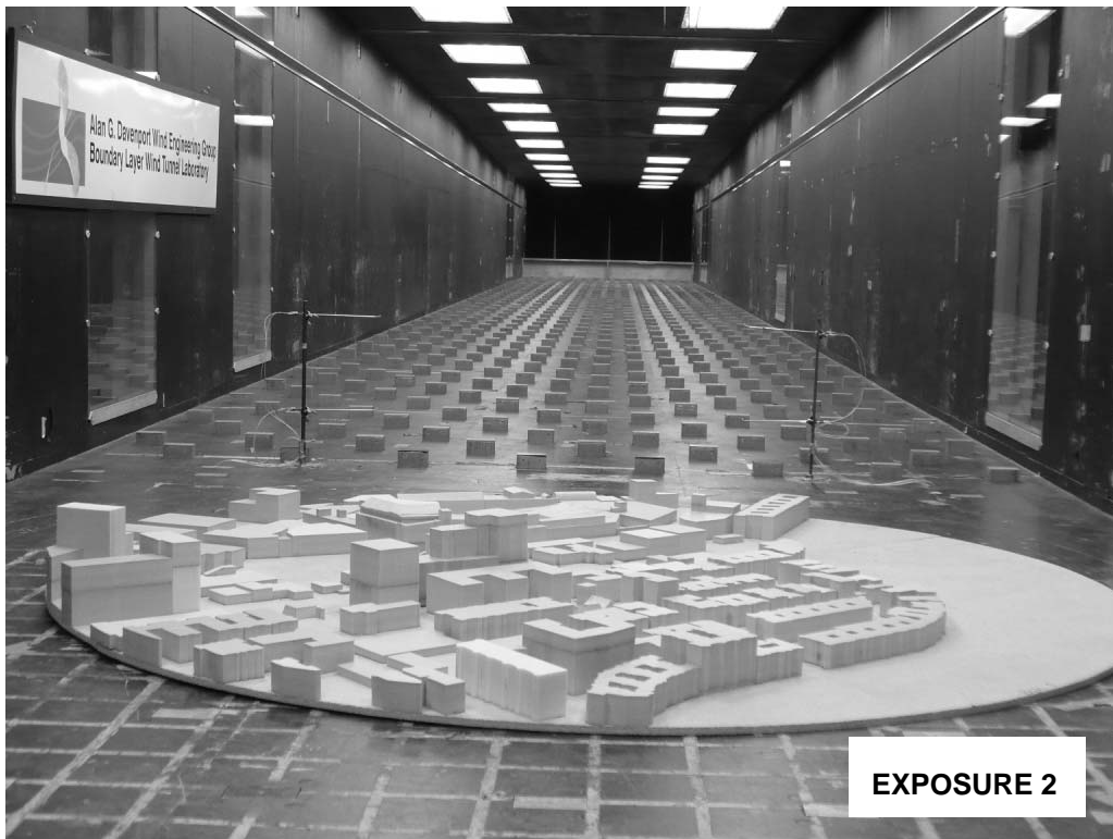
FIGURE 5a PHOTOGRAPHS OF THE MODEL IN THE WIND TUNNEL SHOWING THE UPSTREAM TERRAIN MODELS (EXPOSURES) USED – **BARE SITE CONDITION**
