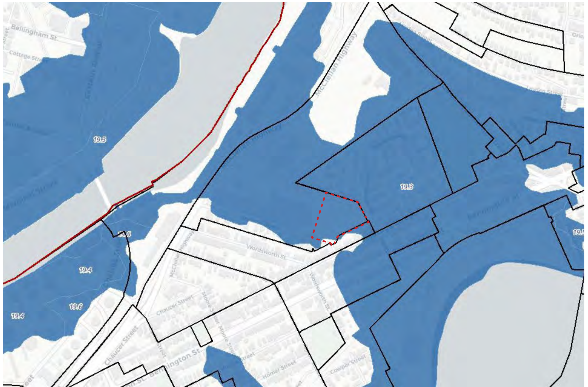
Figure 3-3 Sea Level Rise - Base Flood Elevation Source: Boston Planning & Development Agency, 2018
