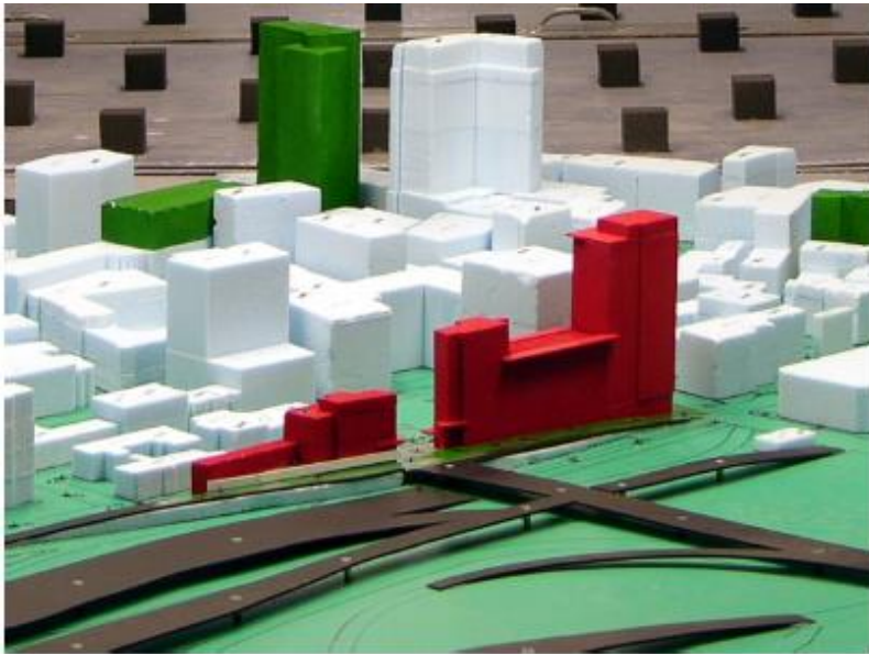
Image 6: Wind Tunnel Study Model for Parcel 24 Project
