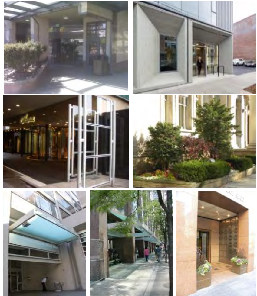
Image 8: Wind Control Examples for Building Entrances
