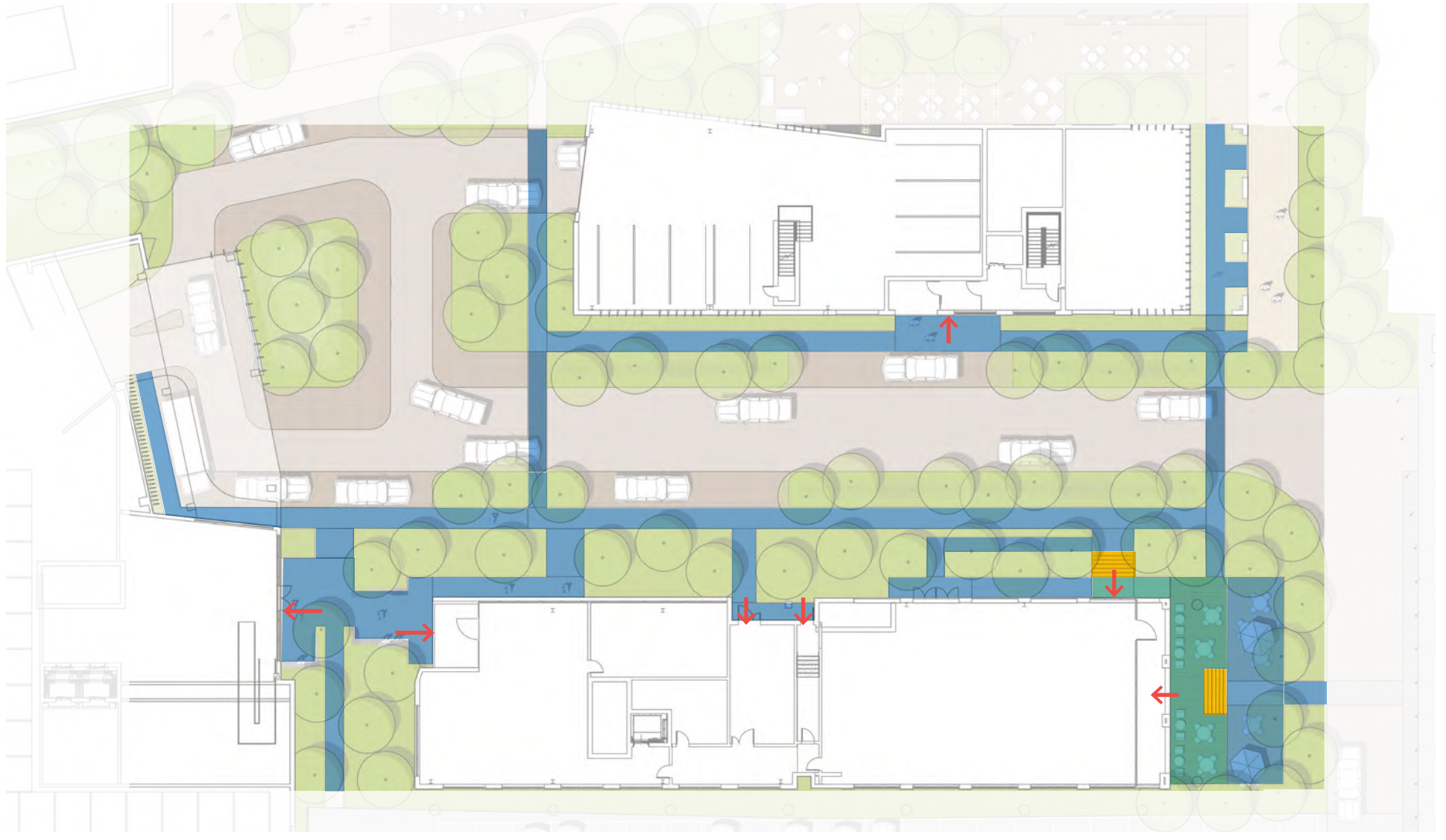
ACCESSIBILITY DIAGRAM - SIDEWALK GRADING
