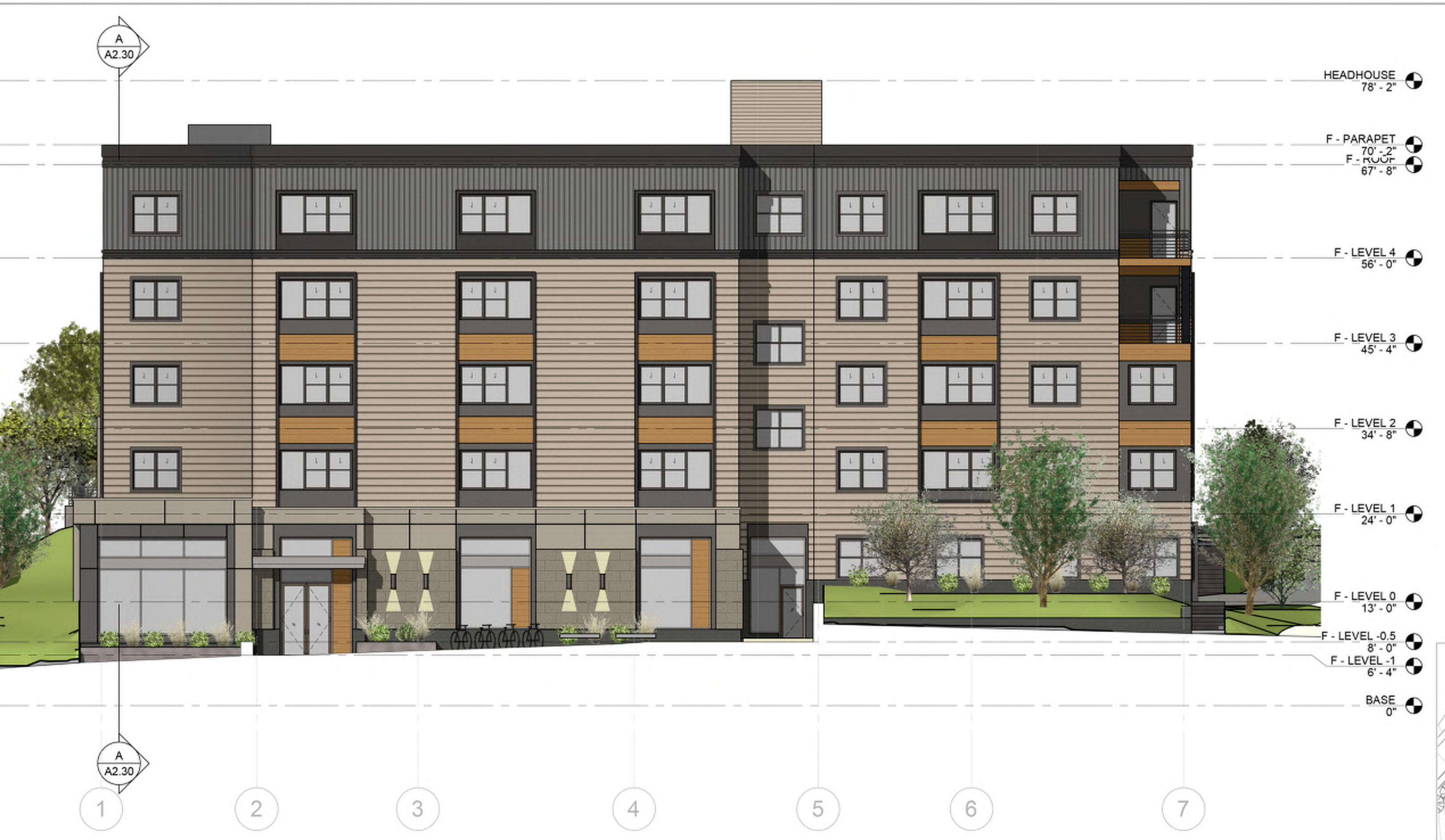
1 BUILDING F - EAST ELEVATION 3/32" = 1'-0"
