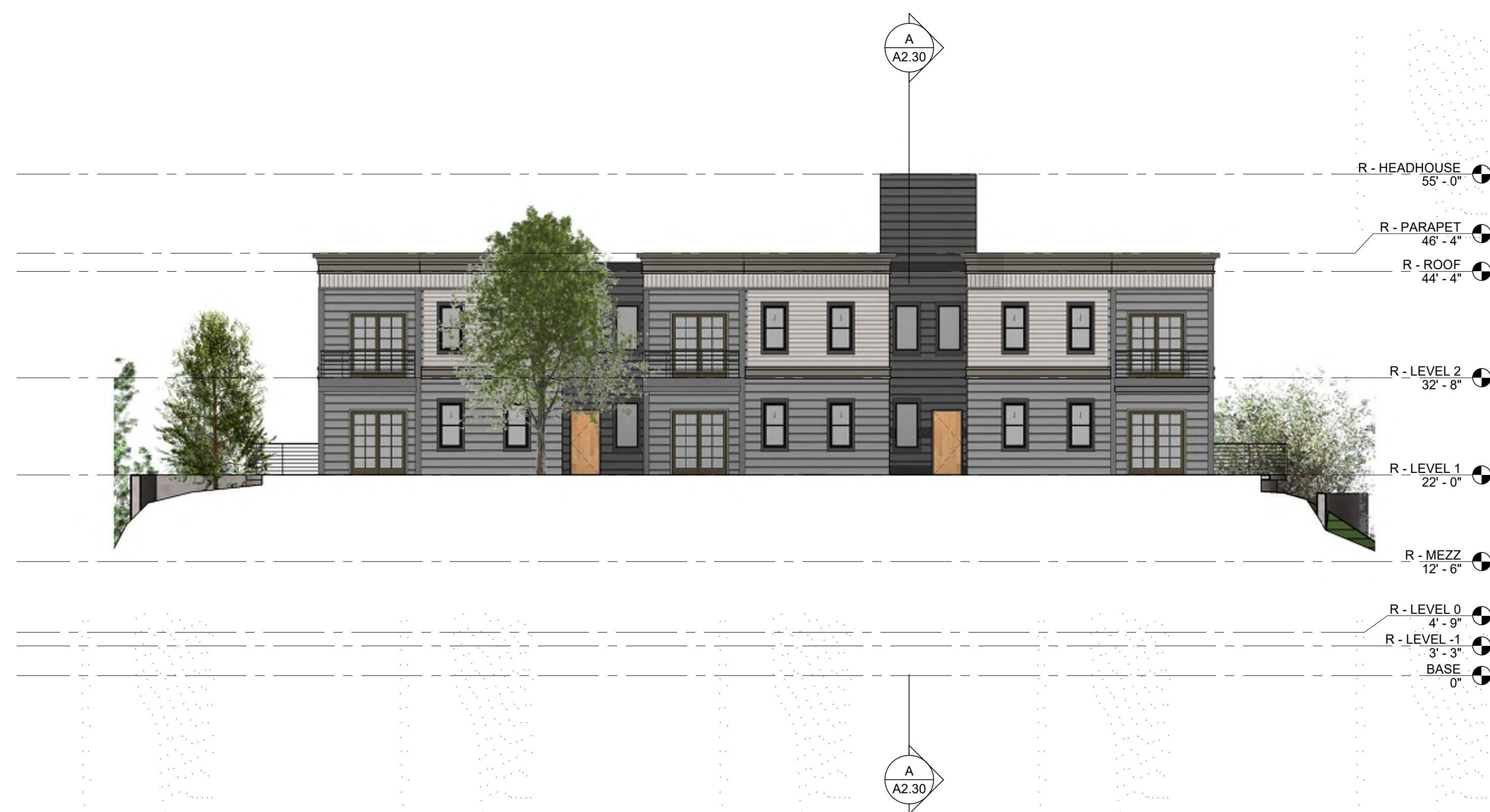
3 BUILDING R - EAST ELEVATION 3/32" = 1'-0"
