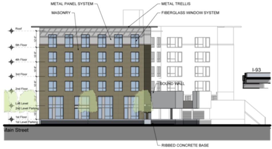
2 North Elevation (JFK Station) SCALE: 1" = 40'
