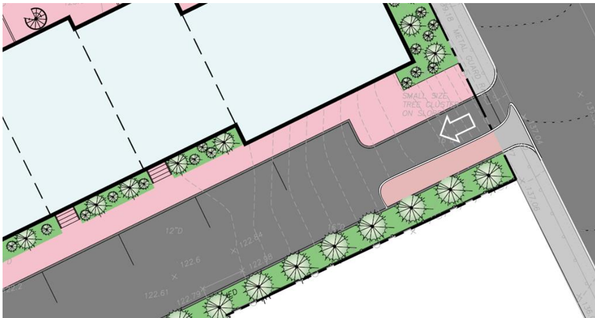
Figure 2.36 – Right-In Driveway Configuration
