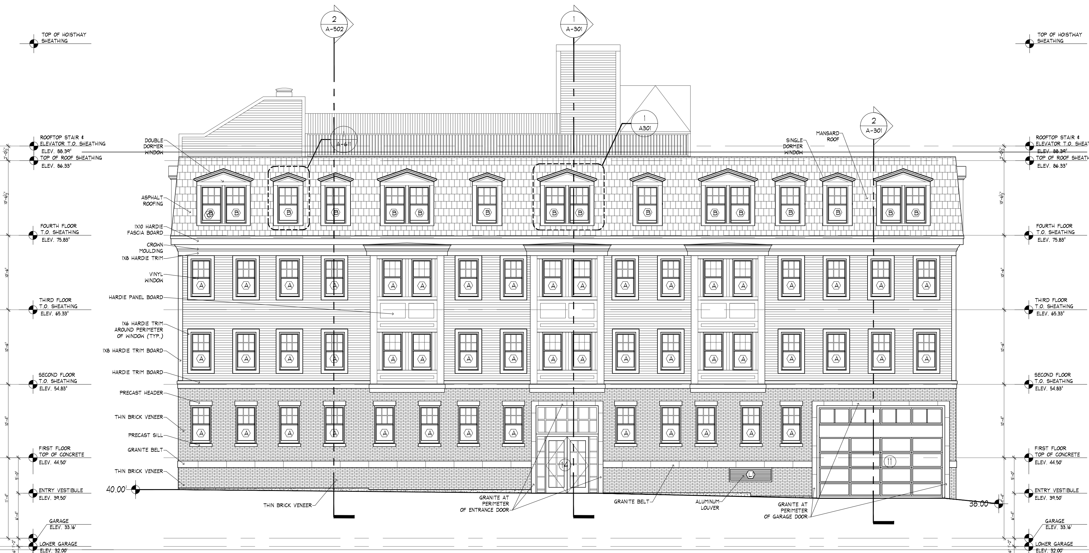
1 ELEVATION FACING POLK STREET SCALE: 1/8" = 1'-0"
