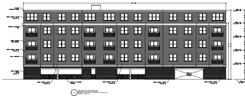
1 REAR ELEVATION SCALE: 1/4" = 1'-0"
