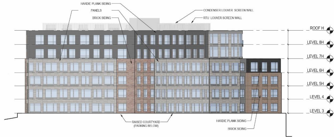
1 ELEVATION - NORTH - COURTYARD 1" = 40'-0"
