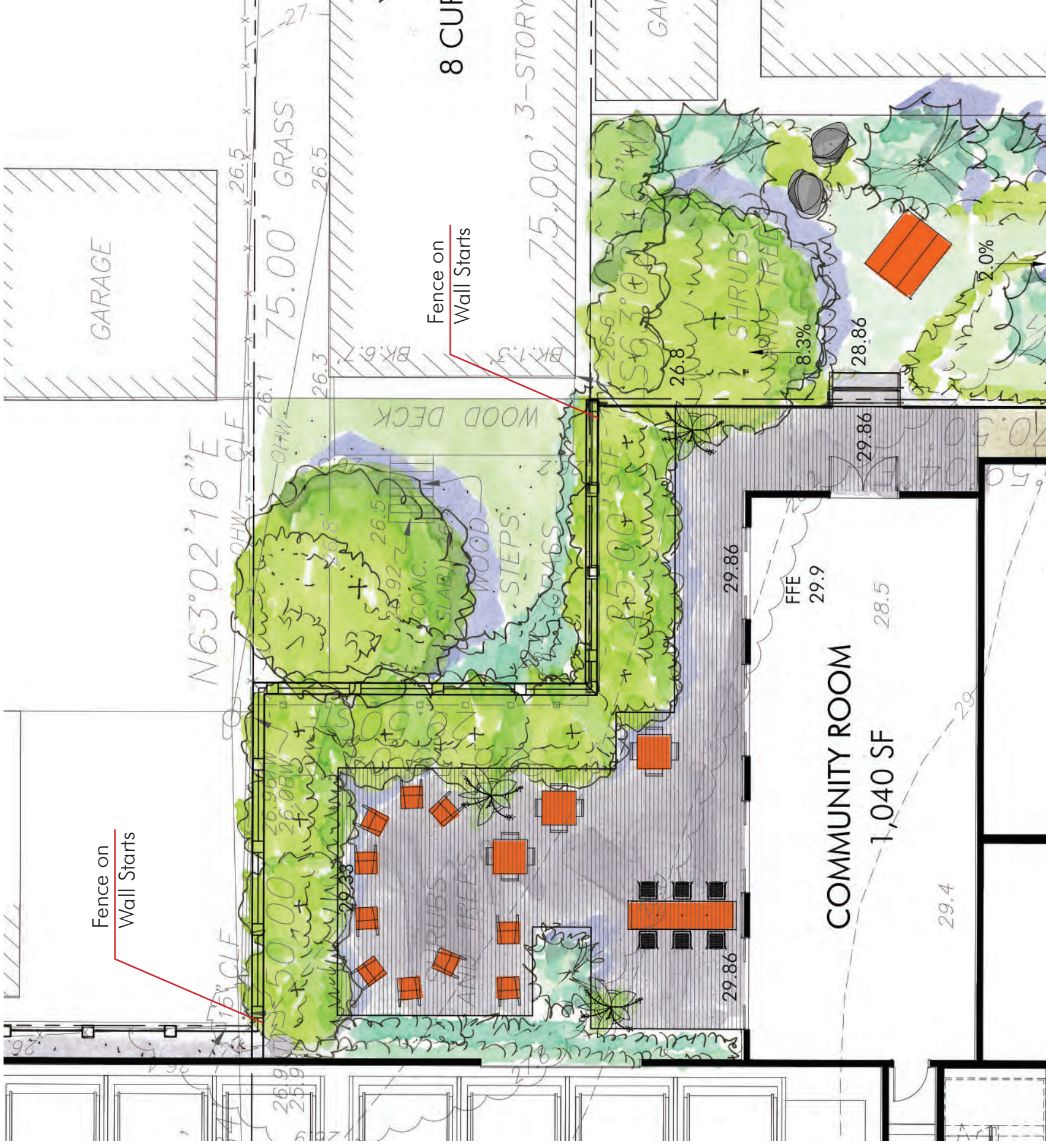
Permeable Pavers define the Rear Yard Terrace allowing infiltration of storm water
