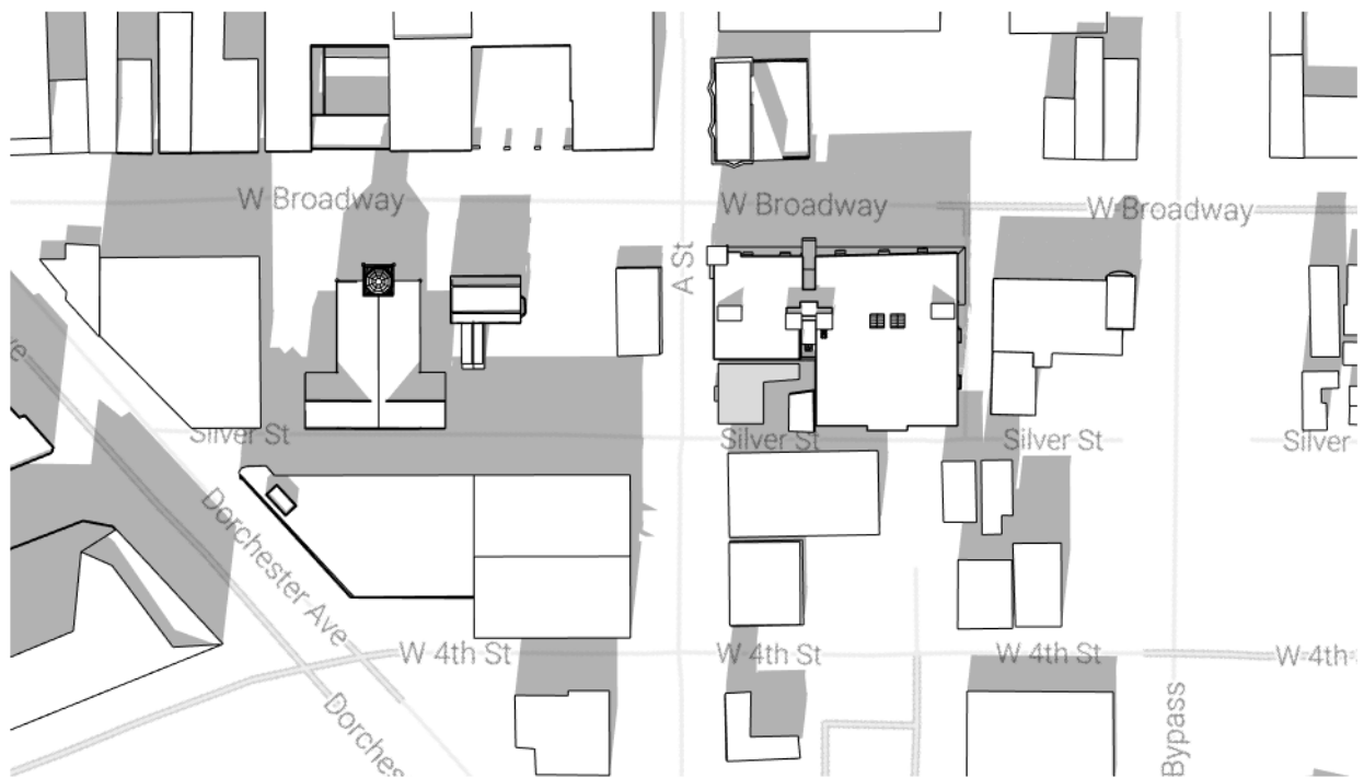
2 Phase: New Construction Sun Date: 9/21 Sun Time: 3PM Sun Altitude: 38° Sun Azimuth: -133°
