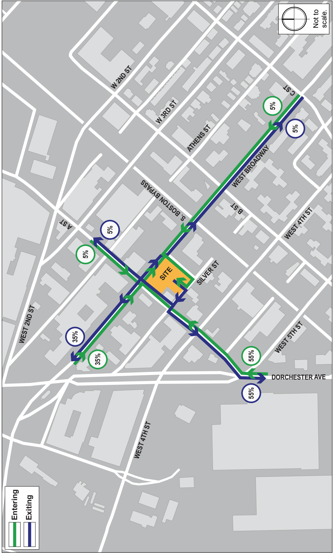
Figure 7-14. Vehicle Trip Distribution
