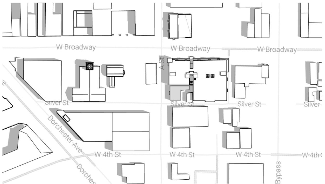
2 Phase: New Construction Sun Date: 6/21 Sun Time: 12PM Sun Altitude: 69° Sun Azimuth: 150°
