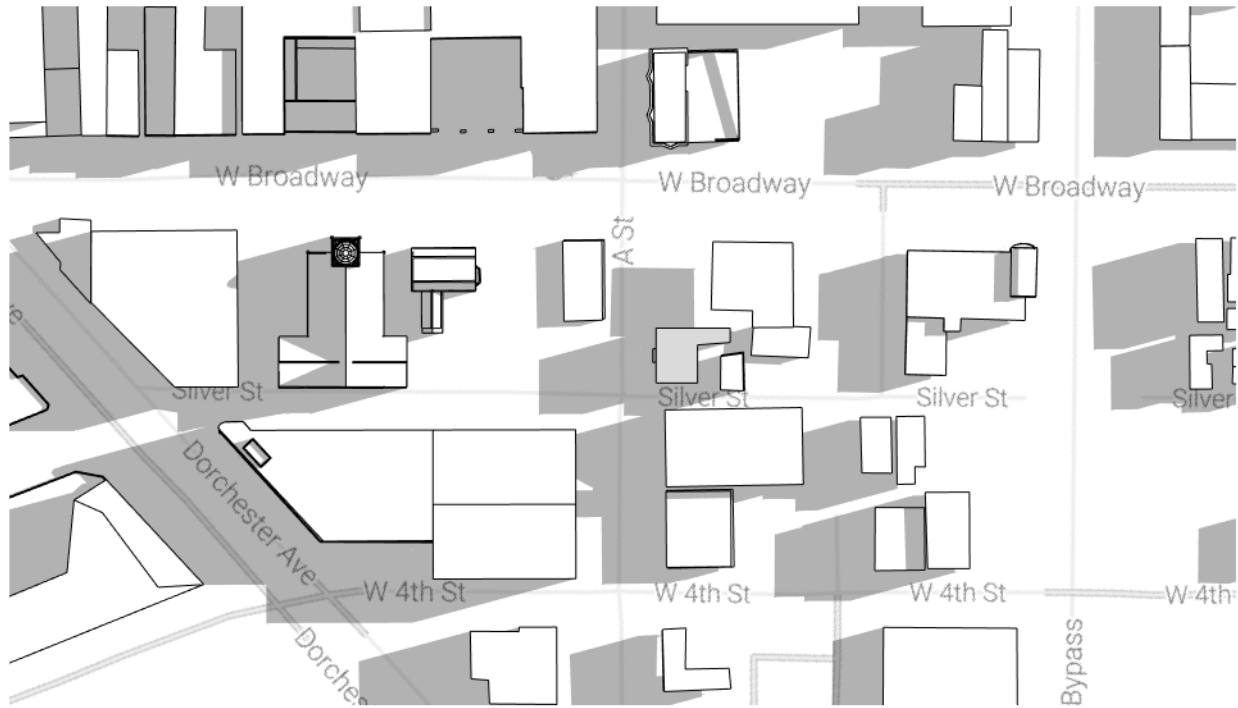
① Phase: Existing Sun Date: 9/21 Sun Time: 9AM Sun Altitude: 26° Sun Azimuth: 115°
