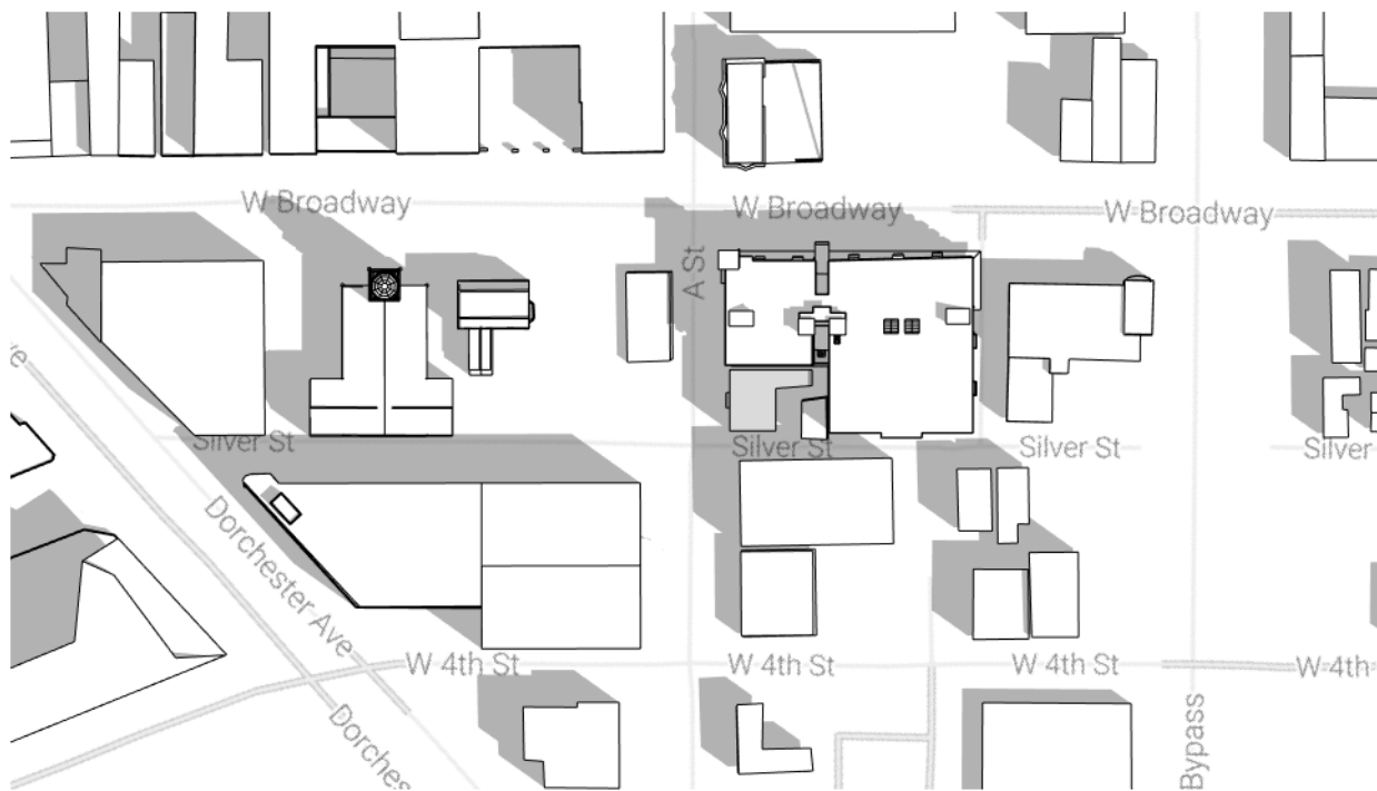
2 Phase: New Construction Sun Date: 9/21 Sun Time: 12PM Sun Altitude: 48° Sun Azimuth: 166°
