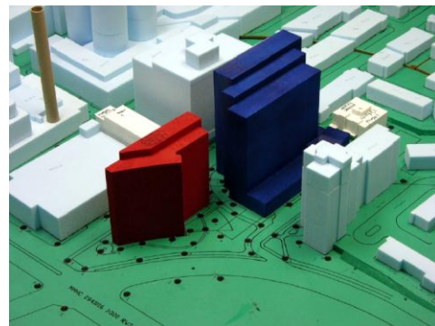
Image 1b – Wind Tunnel Model of Full Build in 2009
