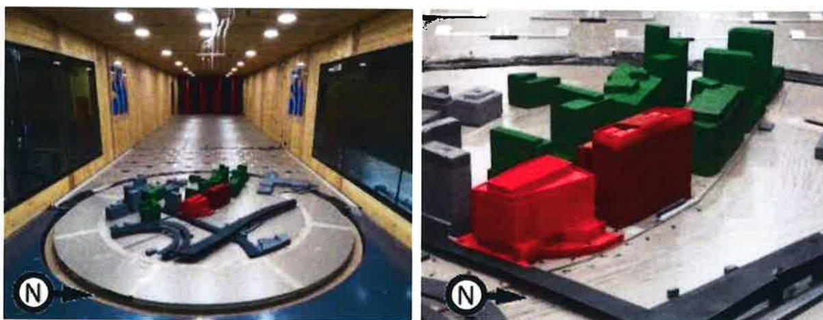
Image 2: Wind tunnel study model - future configuration
