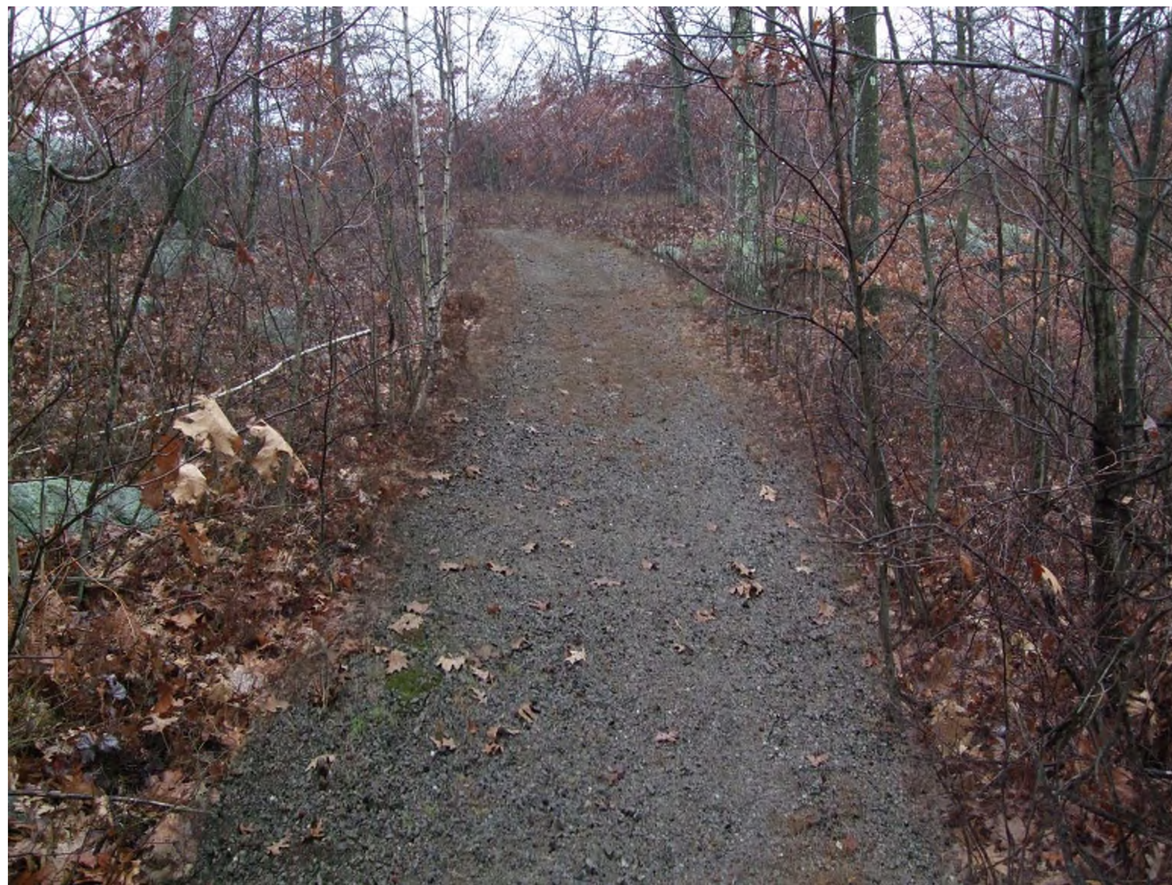
This photo simulation takes the existing trail and shows the desired path width for a Cross Country course – approximately 6-8' wide. The final surface will be a mix of chipped trees and existing gravel from the trail areas. It is the intention of the project to use material from the existing trails and surrounding areas that are disturbed due to the trail width expansion.
