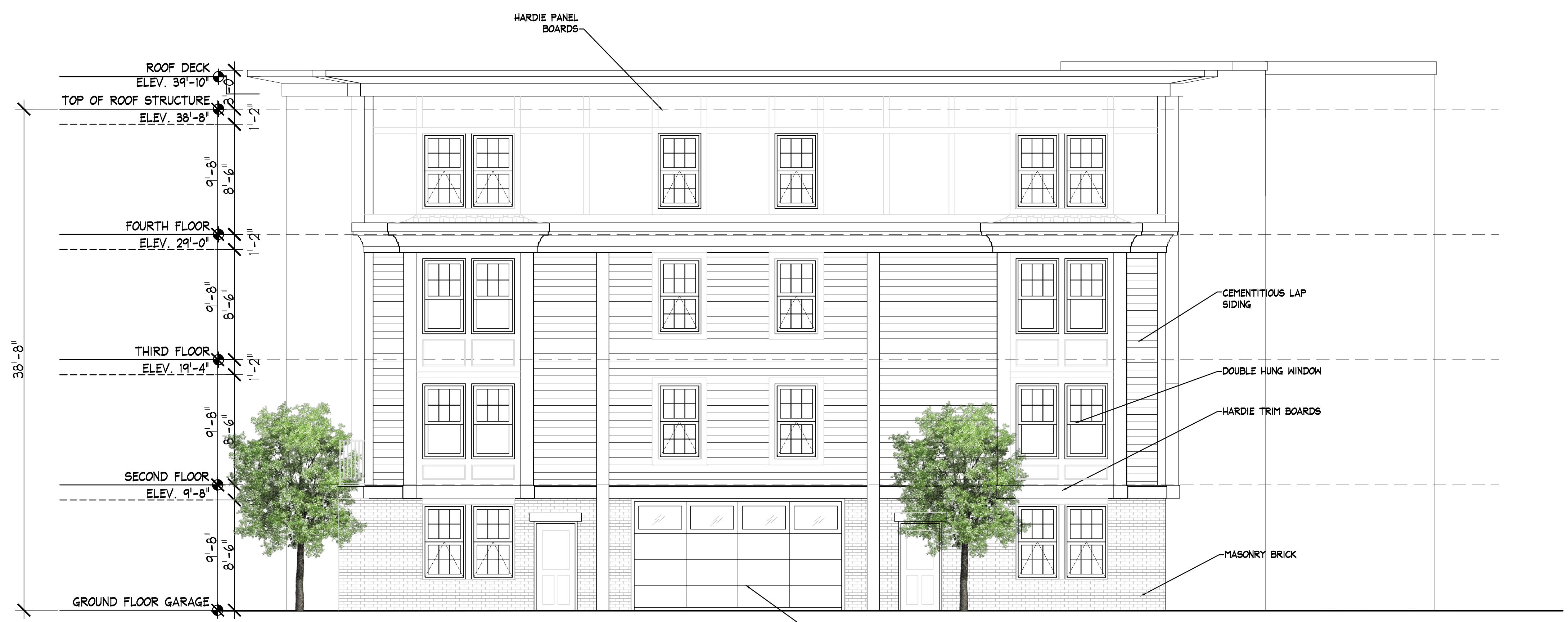
② ELEVATION ON BALDWIN STREET 3/16" = 1'-0"
