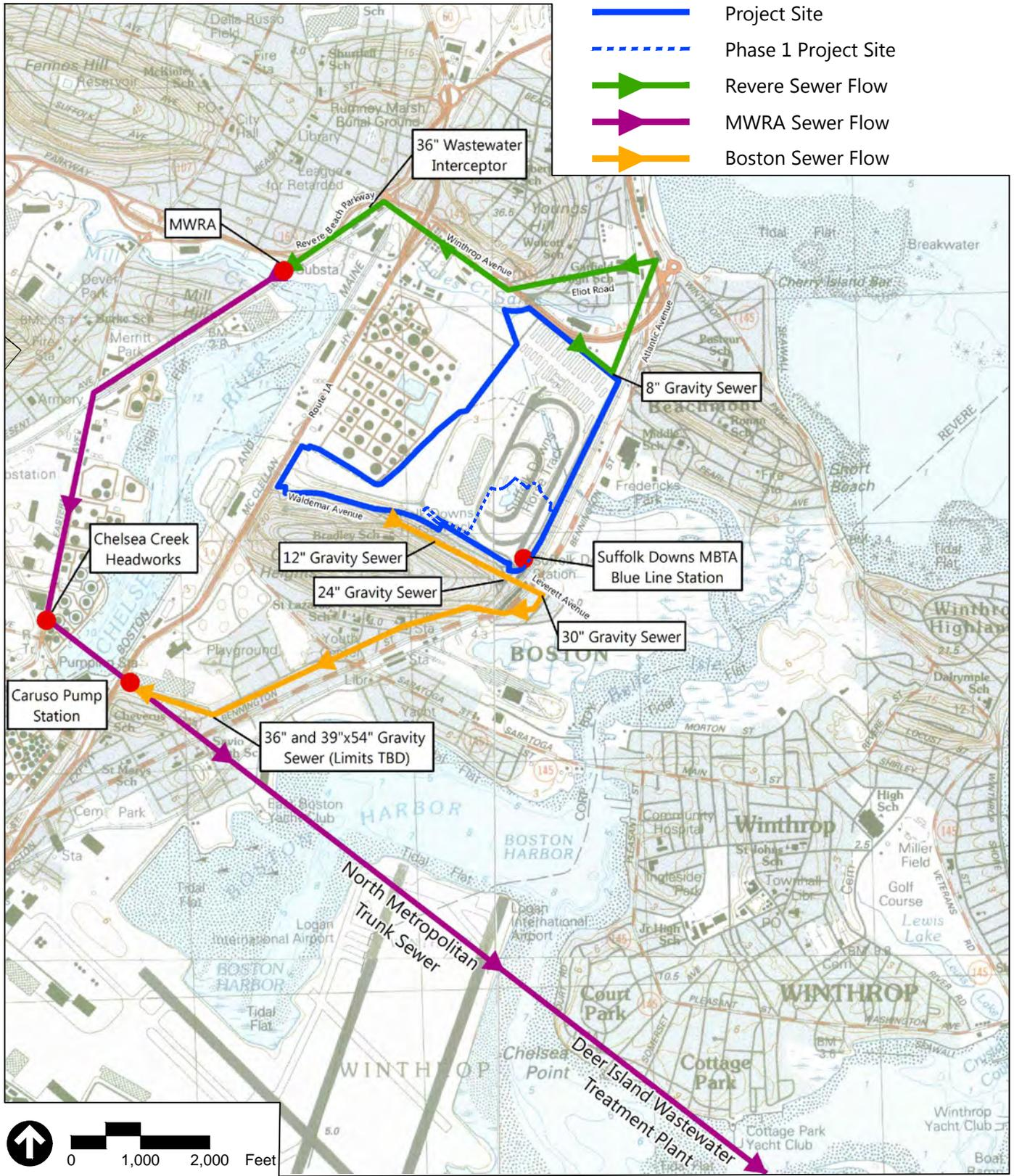
Source: Sewer lines estimated from Environmental Notification Form "Caesars Resort at Suffolk Downs, Boston and Revere, Massachusetts" dated January 31, 2013, EEA No. 15006. Sewer alignments are illustrative and do not necessarily represent actual locations.
